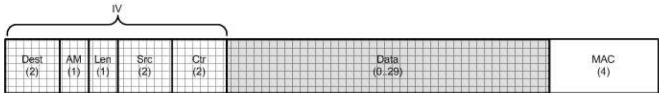
(a) TinySec-AE packet format
