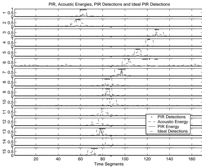
**Fig. 5.** PIR, Acoustic Energies, PIR Detections and Ideal Detections for the 15 sensor nodes of AAV3 data set. It's clear that at later stage the PIR shows false detections for sensor 6, but its negated by Acoustic Modality.
