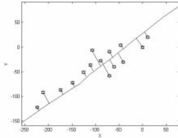
**Fig. 4.** The perpendicular projections of the PIR sensors on to the road
