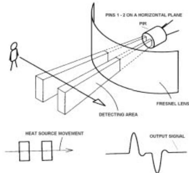
**Fig. 3.** The PIR sensor with the expected output signal
