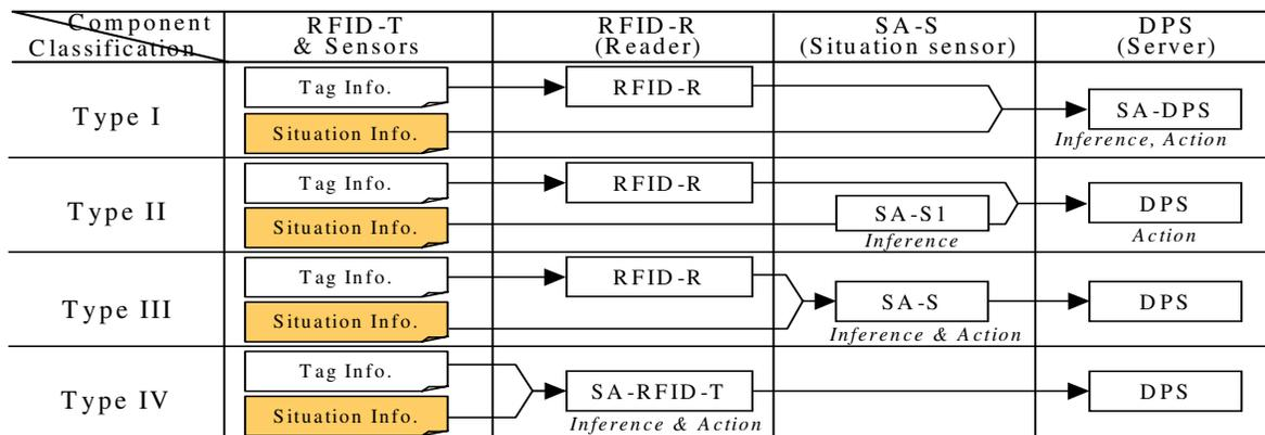
Figure 2. SA-RFID Architectures
