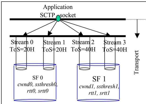
Figure 2: Sub-association Flow Schematic
