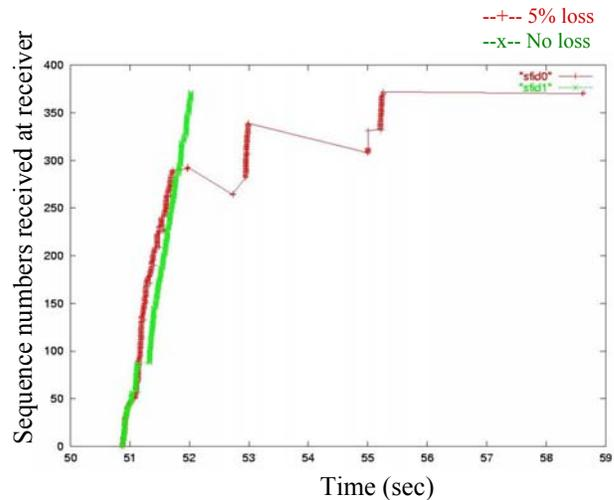
Figure 4: Transfer latency with modified SCTP, and per-stream ToS marking
