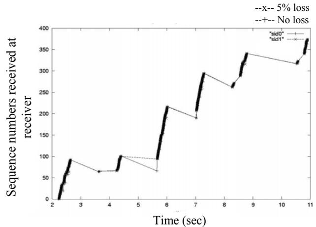
Figure 3: Transfer latency with unmodified SCTP, and per-stream ToS marking
