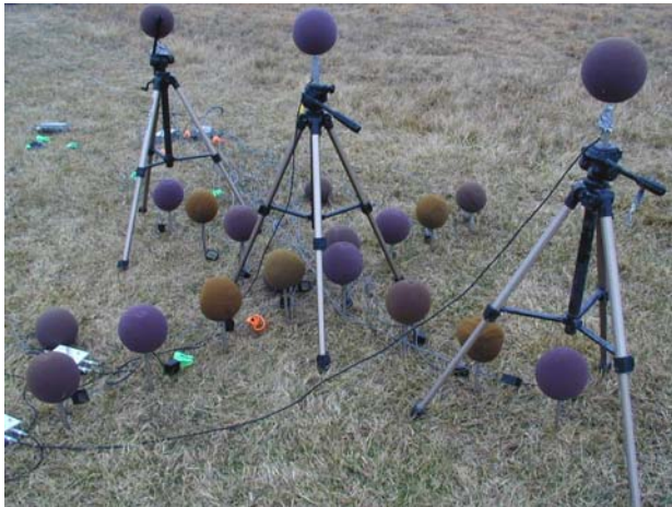
Figure 2: 16-element cross sensor array with 1 foot spacing located on the ground.
