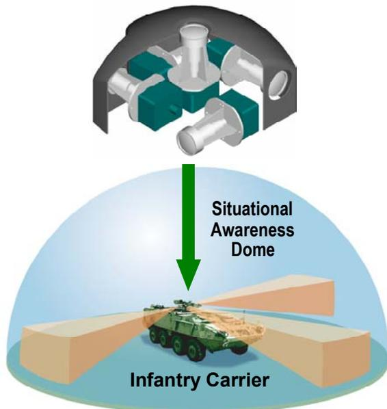
Figure 3 Distributed aperture concept
