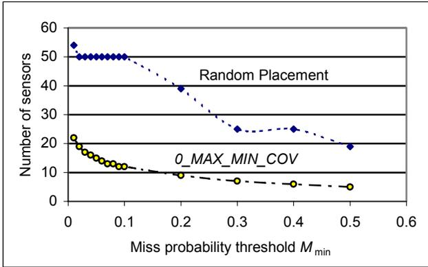
Figure 1: Comparison of  $0\_MAX\_MIN\_COV$  and random placement algorithms for a 20 by 20 grid with randomly placed obstacles.
