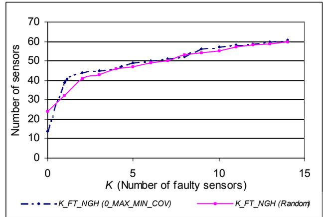
Figure 3: Number of sensors required as a function of number of faulty sensors ( $K$ ) for the  $K\_FT\_NGH$  algorithm.
