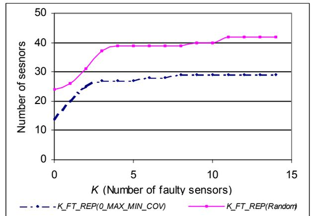
Figure 4: Number of sensors required as a function of number of faulty sensors ( $K$ ) for the  $K\_FT\_REP$  algorithm.
