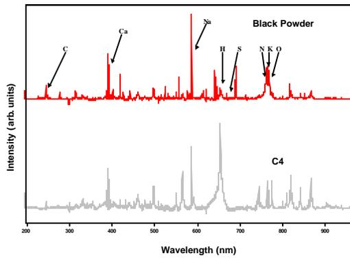
Fig. 1. Single-shot LIBS spectra of C4 and black powder
