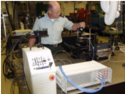
Fig. 3. The new LIBS 2000+ broadband 7-spectrometer detector at ARL
