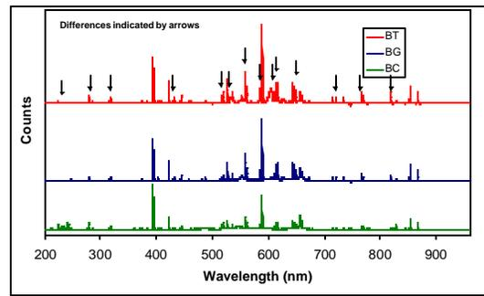
Fig. 2. LIBS spectra of anthrax surrogates BC, BG, and BT
