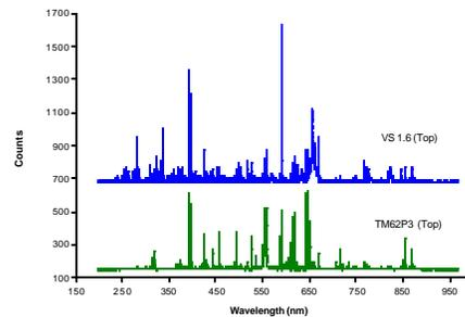
Fig. 4. Single-shot LIBS spectra of plastic casings for the VS 1.6 and TM62P3 landmines
