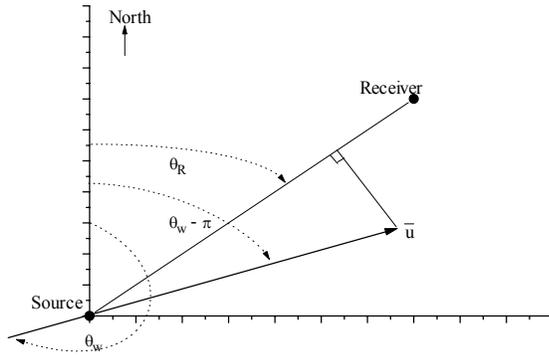
Fig. 6 Geometry schematic for the effective sound speed ( $c_{eff}$ ) that includes the sound speed component due to the mean wind along the path of propagation.
