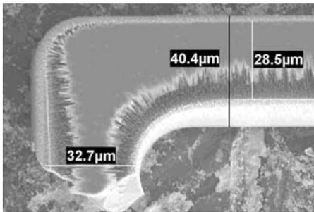
Figure 7. Underside of 40- $\mu$ m spring, showing undercutting.
