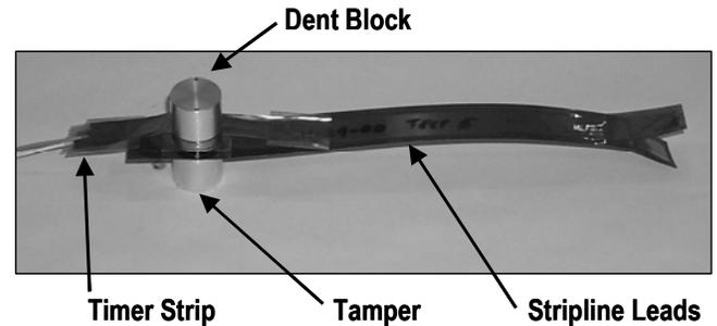
Figure 14. Fixture for MSF test and demonstration.
