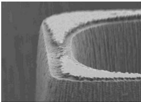
Figure 8. Perspective view of undercut spring.
