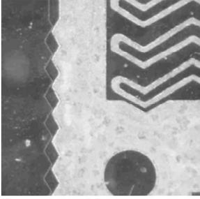
Figure 10. Nickel zig-zag slider mass and spring, with silicon frame and substrate.
