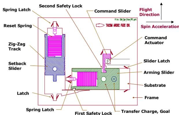
Figure 1. Basic MEMS S&A design, transfer charge in the safe position.
