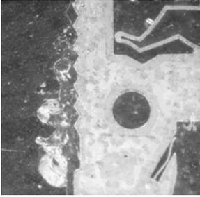
Figure 11. Similar nickel zig-zag slider mass and latch, post-flight.
