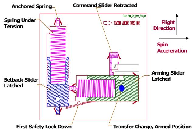
Figure 2. Basic MEMS S&A design, components in the armed position.
