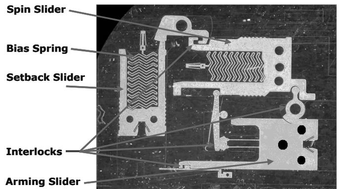
Figure 9. Three-slider, four-lock, 12x15-mm design.
