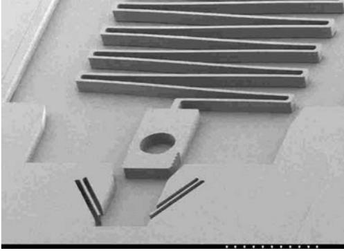
Figure 4. DRIE reset spring bias latch, 100- $\mu$ m thick.
