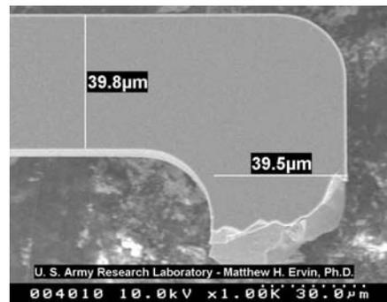
Figure 6. Top of 40- $\mu$ m spring.
