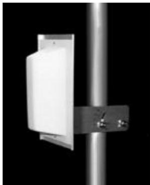
The TA-2404-2-90 is a vertically polarized 90 degree sectoral antenna. It was designed specifically for wireless data and point-to-multipoint radio applications. Radiating elements are protected by a weatherproof radome for operation under severe weather conditions (icing, salt, air, acid rain, etc.) and are at DC ground to aid in lightning protection.
