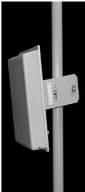
The TA-2408 is a vertically or horizontally polarized panel antenna. The antenna consists of a printed broadband dipole array enclosed in an aluminum cavity with a UV stabilized ASA radome for superior weatherability. It is designed for wireless data in the ISM band and is at DC ground to aid in lightning protection.
