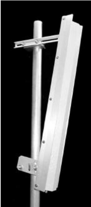
The TA-2405H-2-45 is a high gain 45 degree horizontally polarized sectoral antenna consisting of a broadband dipole array mounted on a solid aluminum reflector and covered with a weatherproof radome. The antenna was designed for operation under severe weather conditions and is at DC ground to aid in lightning protection.
