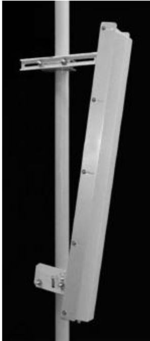
The TA-2304-2-ISM is a vertically polarized sectoral antenna which has adjustable side panels for 60-160 degree azimuth patterns. The antenna consists of a printed dipole array enclosed in an aluminum base with a UV stabilized radome for superior weatherability. It is designed for wireless data in the ISM band and is at DC ground to aid in lightning protection.
