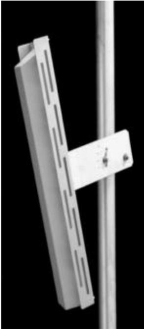
The TA-2404-4-60 is a vertically polarized 60 degree sectoral antenna. It was designed specifically for wireless data and point-to-multipoint radio applications. Radiating elements are protected by a weatherproof radome for operation under severe weather conditions (icing, salt air, acid rain, etc.) and are at DC ground to aid in lightning protection.
