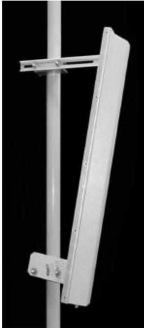
The TA-2304-2-180-ISM is a vertically polarized sectoral antenna with a fixed 180 degree pattern. The antenna consists of a printed dipole array enclosed in an aluminum base with a UV stabilized radome for superior weatherability. It is designed for wireless data in the ISM band and is at DC ground to aid in lightning protection.
