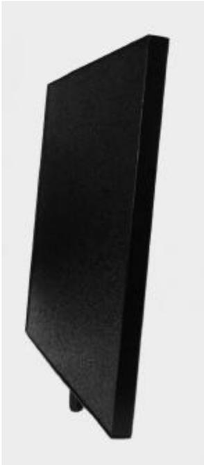
The TA-2407P is a compact, light-weight, vertically polarized panel antenna intended for mounting onto the back of a laptop computer for special applications in the ISM band. The antenna consists of a printed patch array enclosed in a black painted aluminum cavity with a black UV stabilized ASA radome.
