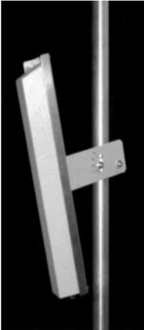
The TA-2404-4-90 is a vertically polarized 90 degree sectoral antenna. It was designed specifically for wireless data and point-to-multipoint radio applications. Radiating elements are protected by a weatherproof radome for operation under severe weather conditions (icing, salt air, acid rain, etc.) and are at DC ground to aid in lightning protection.
