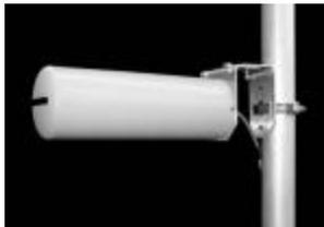
The TA-2411 is a vertically or horizontally polarized yagi antenna. The antenna consists of a printed broadband yagi enclosed in a UV stabilized ASA radome for superior weatherability. It is designed for wireless data in the ISM band and is at DC ground to aid in lightning protection.
