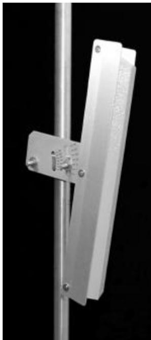
The TA-2304-45-ISM is a vertically polarized sectoral antenna with a fixed 45 degree pattern. The antenna consists of a printed dipole array enclosed in an aluminum base with a UV stabilized radome for superior weatherability. It is designed for wireless data in the ISM band and is at DC ground to aid in lightning protection.
