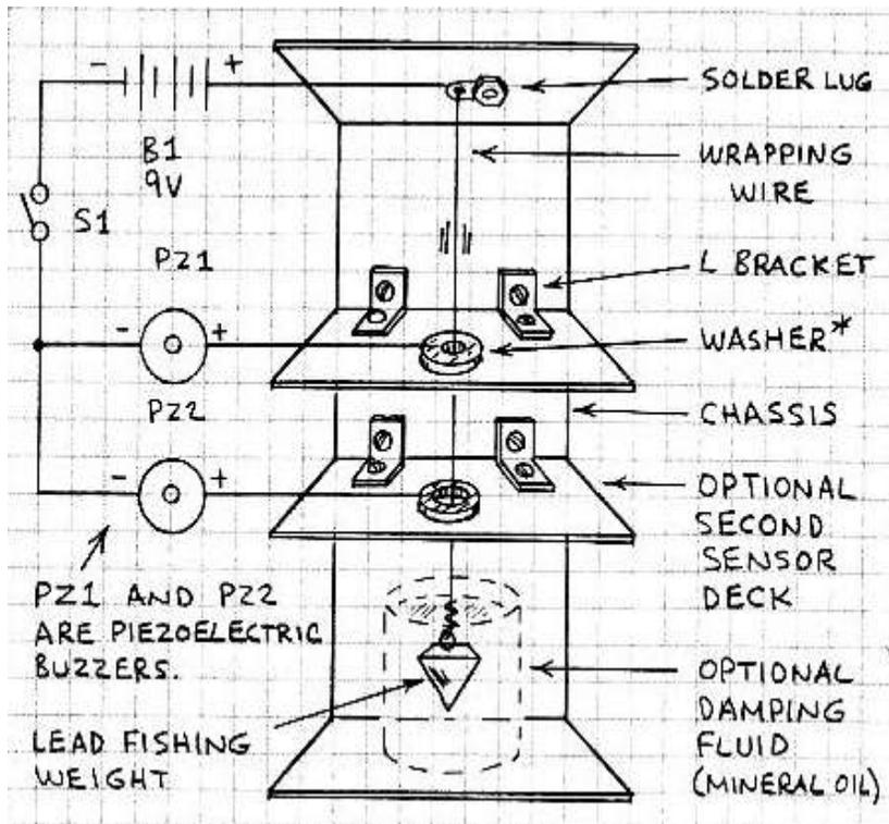
Pendulum switches detect tilt/vibration. Above circuit is simple binary switch, or replacing the sensor ring (washer) with a circular array of four or more segments allows for determination of the direction of tilt or vibration, seen in pendulum quadrant switch circuit to the right.
