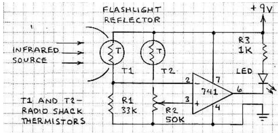
Power circuit and wait a few seconds for thermistors to stabilize, then adjust R2 until LED just switches off. Placing hand near reflector should trigger circuit, a lit match will trigger it from about 3 feet or more.
