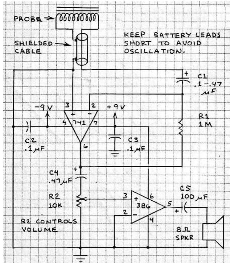
Test the probe by placing near a telephone receiver. Should hear dial tone when phone is off the hook.
