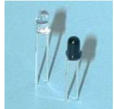
Note that phototransistors may or may not have a base lead (if they do, the base lead allows you to bias the phototransistor's light response).
